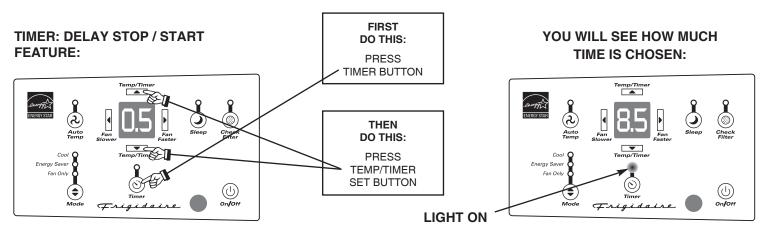
**Note 1:** For Delay Stop, the unit must be in the On position. **Note 2:** For Delay Start, the unit must be in the Off position.
